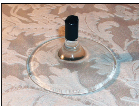
Fig. 3. The "gravitational" lens. The lens is a broken off wine glass base. For safety, we smoothed the stem's top with a Dremel tool and placed black tape over the rough edge. Additionally, this tape serves a scientific purpose: it blocks visibility down the center of the glass. For a cluster or other massive and luminous lensing object, background sources are not generally visible down the center of the gravitational lens.
