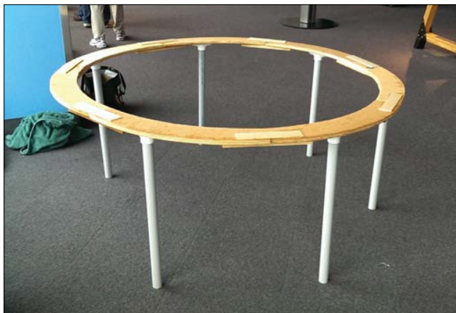
Fig. 4. The circular wooden frame of the gravity simulator. The simulator stands 3 ft tall and the inner diameter is about 5 ft.
